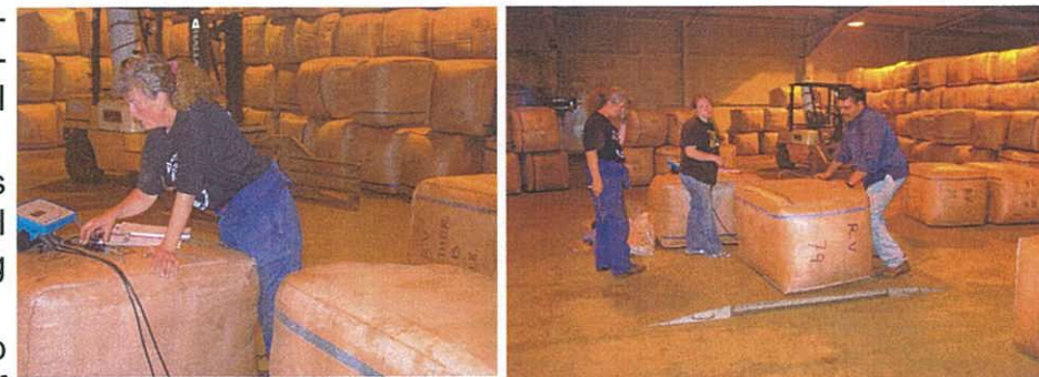
Core Sampling at the Wool Warehouse
