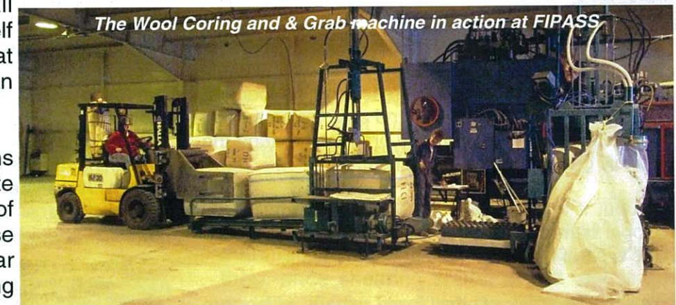
Step 3 - compress and core the bales
