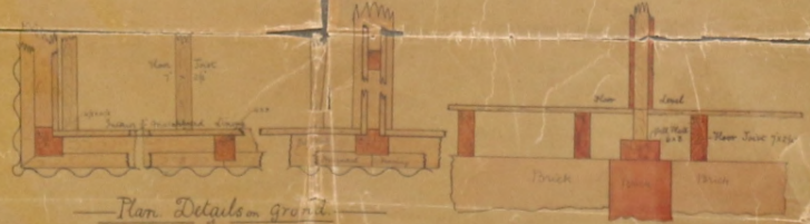
Corner Joint Framing Joint Partition Joint Section of Partition Joint Scale 1/4" = 1'
