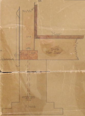
Section of Base of Building Scale 3/16
