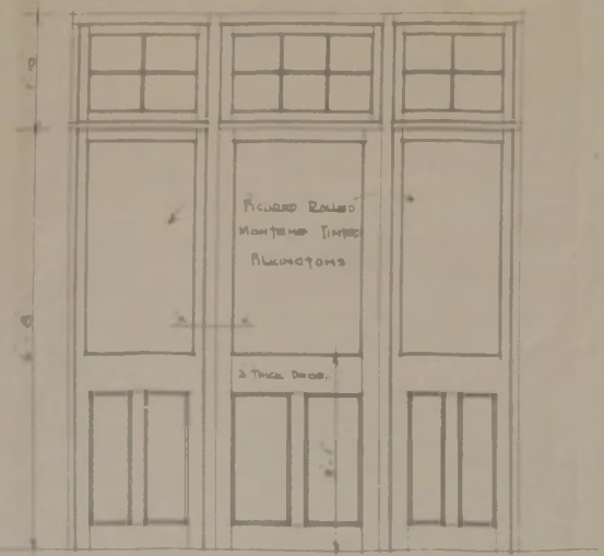
~ ELEVATION ~ OF ~ DOORS ~ TO ~ HALL ~ FRONT ~ 1 DOOR ONLY AS ABOVE 68-28 TO HALL SIDE
