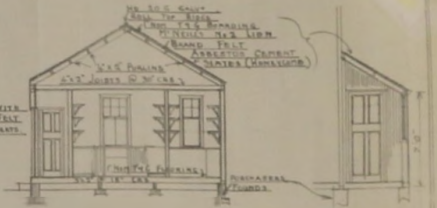
~ SECTION - THRU - SCULLERY - PANTRY -
