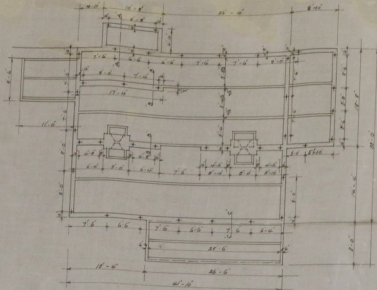
~ FOUNDATION & ANCHOR BOLT PLAN ~
