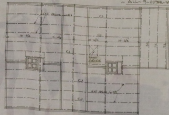
~ PLAN OF CEILING JOISTS ~
