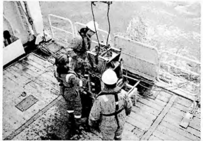
A box corer is deployed to retrieve benthic samples - benthic data is used to form an Environmental Baseline Survey, which in turn forms part of a company's EIA (Picture: RPS Energy)
