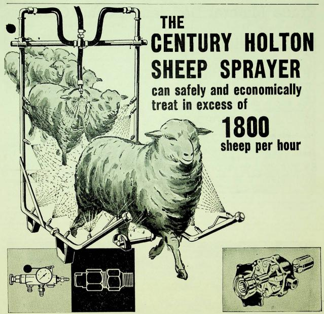
ACCURATE POSITIVE 20 BRASS NOZZLES WITH PRESSURE CONTROL UNIT SET SPRAY PATTERN
