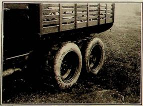
As can be judged from the photograph, the chains are laid out on the ground and the vehicle is backed over them. Each chain is then joined as in the left-hand photograph.
