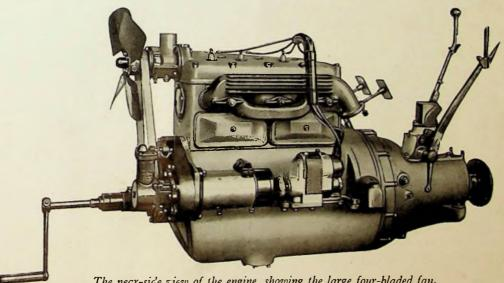
The near-side view of the engine, showing the large four-bladed fan, water impeller in the cylinder head, engine-driven tyre pump and the tandem mounting of the dynamo and magneto. The manifolding, too, is particularly neat, affording ample flow for the ingoing gases and freedom for the exhaust.
