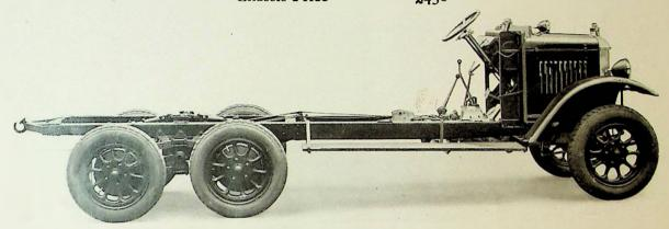
Both 30-cwt. and 2-ton models may be equipped with either  $33'' \times 5''$  single tyres or  $32'' \times 4\frac{1}{2}''$  twins on driving axles, with the option of  $32'' \times 6''$  singles all round at an extra cost of £50.
