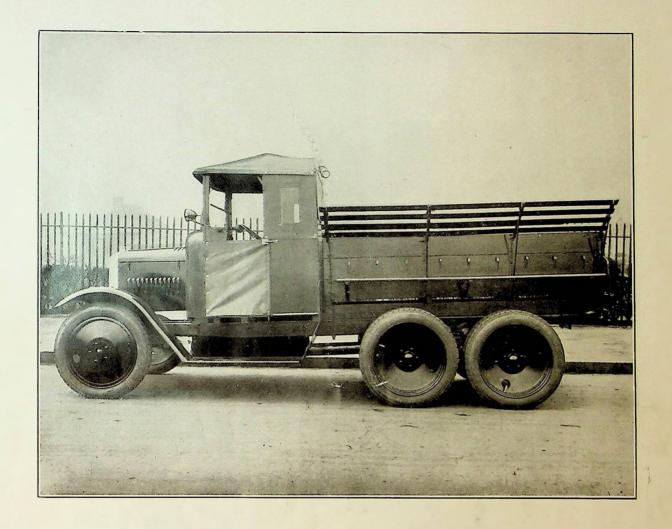
The 30-cwt. Model with War Office Type Body Mounting Although its performance is very much out of the ordinary there is nothing grotesque or particularly unusual in the appearance of the complete Morris-Commercial Six-Wheeled Vehicle. The rear wheels are mounted as close together as can conveniently be arranged, so that mudguarding is an easy matter, while the driver's cab does not depart from the usual practice.
