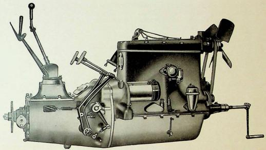
From this off-side view of the engine it will be appreciated that the layout of all components is particularly neat, and extreme accessibility can be claimed for oil filling arrangements and also for carburetter.
