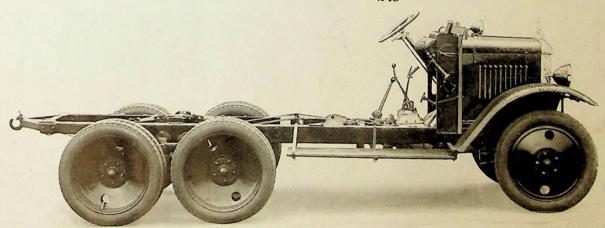
The frame itself is of sturdy dimensions, capable of withstanding the hardest usage. Ample body space is allowed. The rearmost gear lever controls the two-speed epicyclic gear which augments the four ratios provided by the normal gearbox. The whole chassis is robust and thoroughly reliable, a remarkable example of an efficient vehicle sold at a reasonable price.
