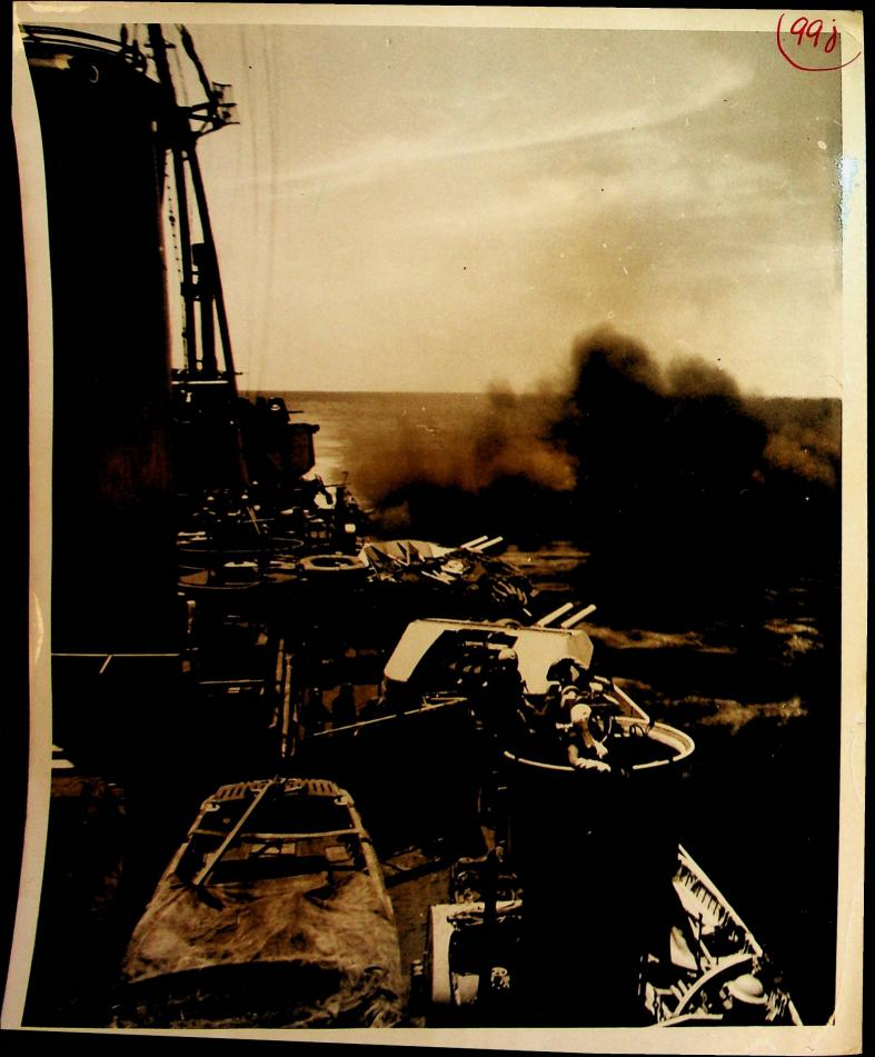
Guns of H.W.C.S. "UGANDA" boom out against the Sakishima islands, south of Okinawa, during a British Pacific Floet bombardment. Smoke is not coming from the guns visible in the picture, which are anti-aircraft, but from the six-inch battery aft.
