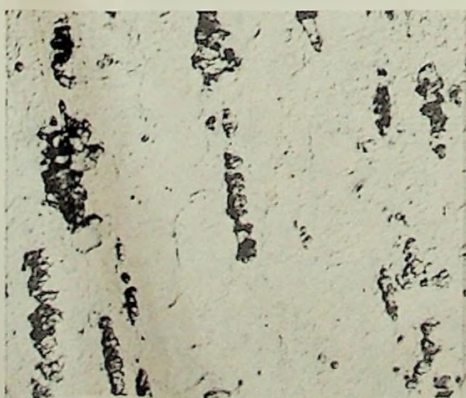
Figure 1 Intermetallic particles of yttrium after cold rolling
