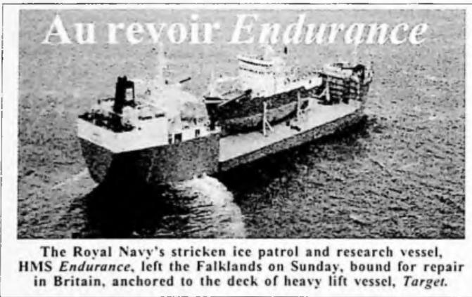
The Royal Navy's stricken ice patrol and research vessel, HMS *Endurance*, left the Falklands on Sunday, bound for repair in Britain, anchored to the deck of heavy lift vessel, *Target*.
