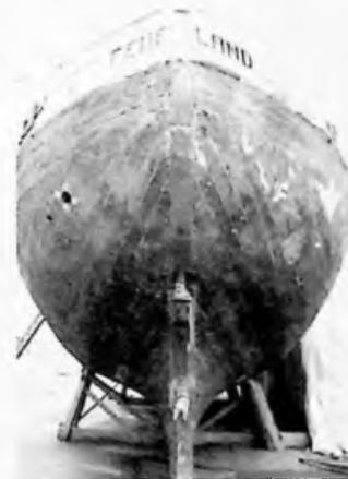
Years and layers of paint stripped away to reveal the hull still in good shape
