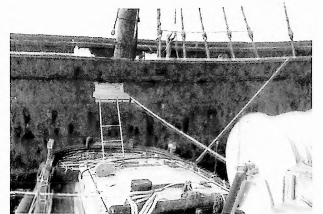
A hole caused by rust in the side of the Lady Liz
