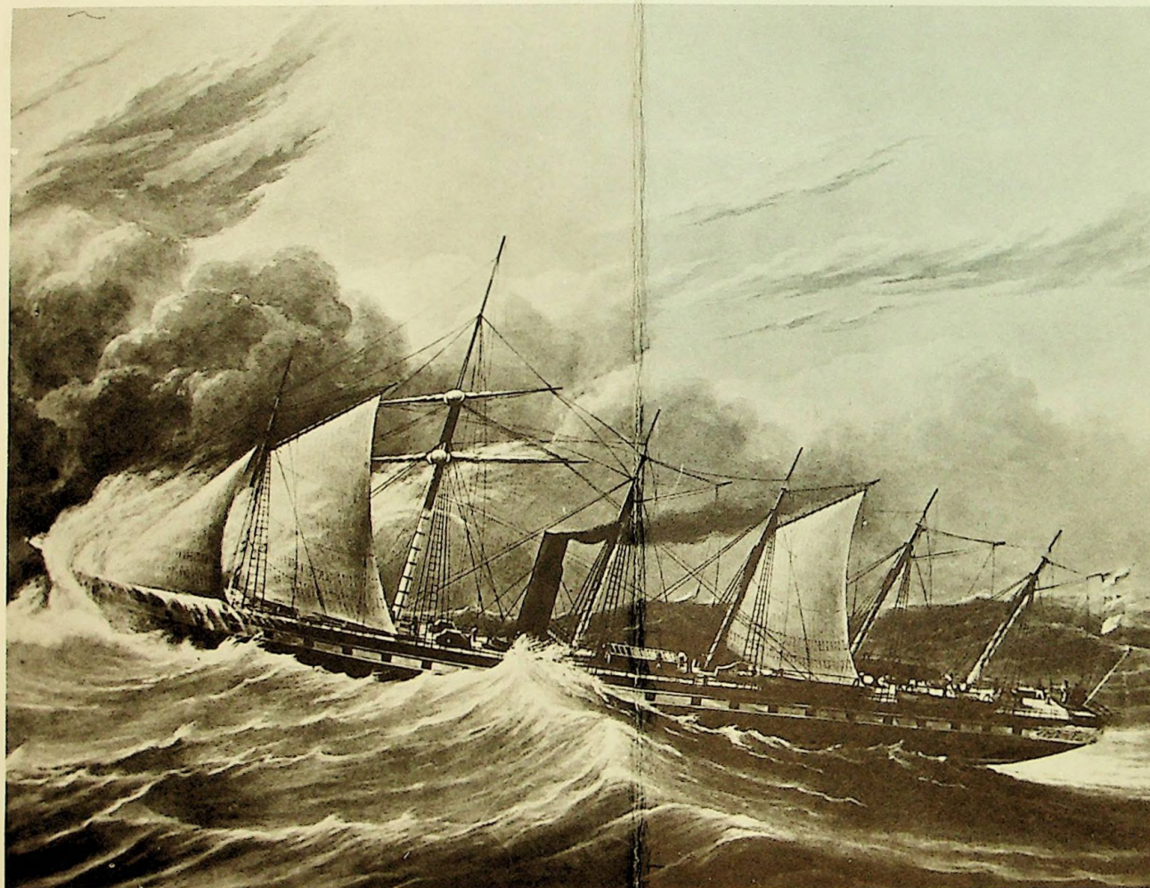
With both sails and a powerful engine, the ss 'GREAT BRITAIN', the first large iron ship, the first ocean-going vessel to be propeller-driven, quickly proved her worth in both rough and calm weather. She best represents the bridge between the days of sail and those of power.
