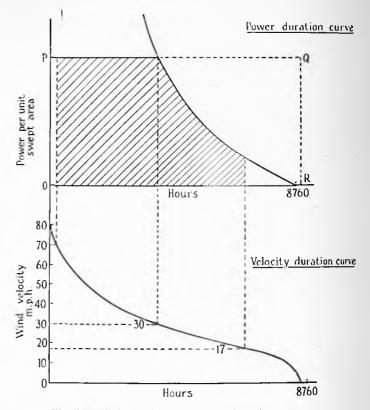
Fig. 7.—Wind velocity and power duration curves.
