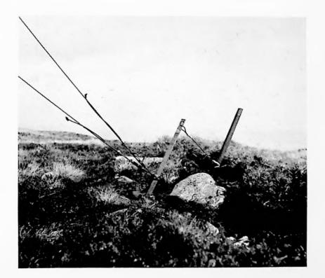
Fig. 2.—Double-picket anchorage.
