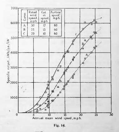
curves which enter into the output calculations with the 30 m.p.h. rated speed.
