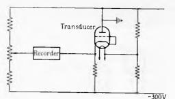
Fig. 7.--Circuit used with the prototype gust-anemometer.
