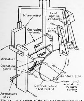
Fig. 33.—A diagram of the dividing mechanism used with the E.R.A. impulse recorder, Series 3.
