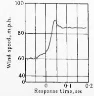
Fig. 12.—Section of chart to show the response of the new prototype anemometer.
