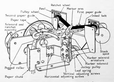
Fig. 32.—Construction of E.R.A. impulse recorder, Series 2.
