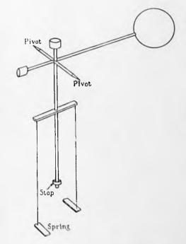
Fig. 15.—Diagram to show the principle of the anemometer for obtaining the vertical component of the wind.
