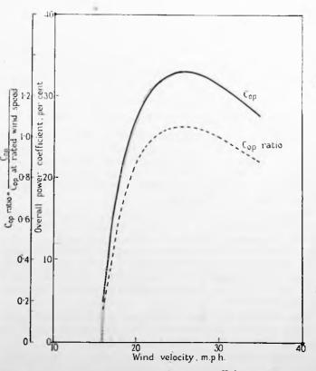
Fig. 18 .-- Curve of overall power coefficients.
