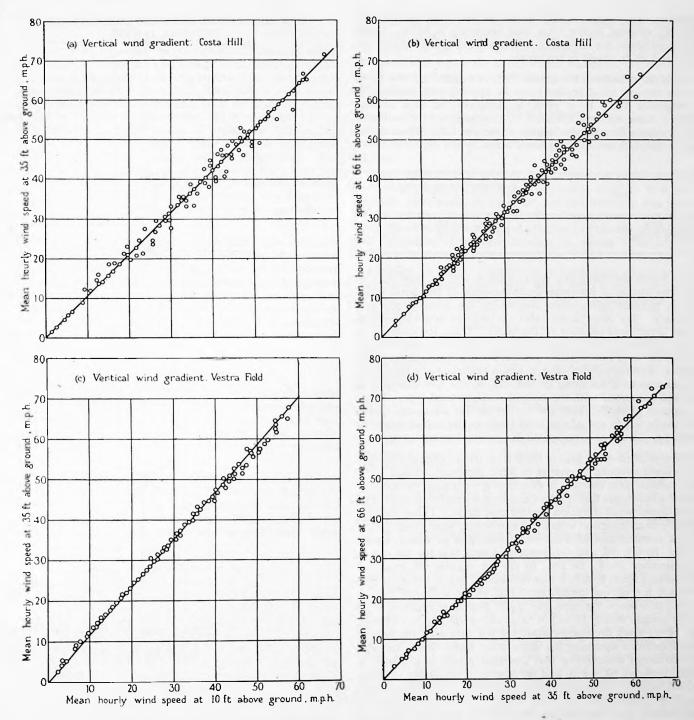
Fig. 15 (a) and (b).—Vertical wind gradient—Costa Hill (35 ft.—10 ft. and 66 ft.—35 ft.). (c) and (d).—Vertical wind gradient—Vestra Fiold (35 ft.—10ft. and 66 ft.—35 ft.).
