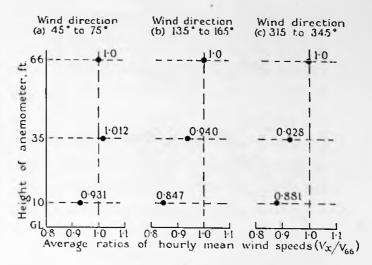
Fig. 20.—Variation of wind speed with height for three wind directions over Costa Hill.
