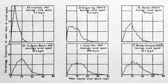
Fig. 10.-Wind velocity/frequency curves for six typical E.R.A. sites (approximately yearly periods).
