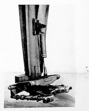
Fig. 3 The damper gear which is mounted on each of the three arms of the hub controls blade movement in the drag plane; the blades themselves act as dampers in the coning plane.
