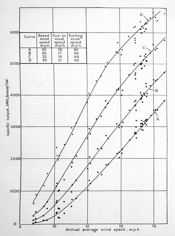
Fig. 17.-Relationship between the specific output and annual average wind speed at sites in the British Isles.
