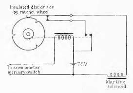
Fig. 3.-Circuit diagram of the contactor mechanism.
