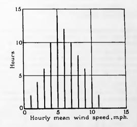
Fig. 12.—A simple velocity/frequency histogram. This figure is usually drawn as a smooth curve.
