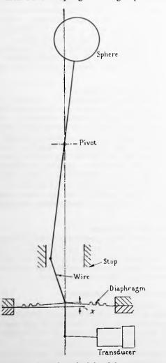
Fig. 4.—Diagram to show the principle of the gust anemometer.
