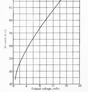
Fig. 5.—Calibration curve of the prototype gust-anemometer.
