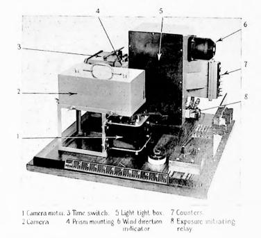
Fig. 3.—Photographic recorder developed for use in the Orkney wind survey.
