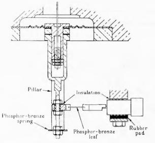
Fig. 8.—Modification of the transducer mounting and lower anchorage.
