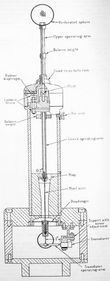
Fig. 6.-Section of gust anemometer.
