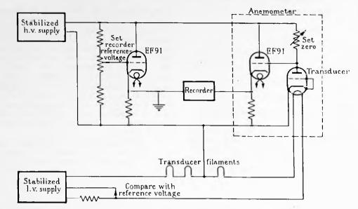
Fig. 10.-Modification of the anemometer recording-circuit.
