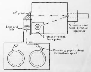
Fig. 1.—Diagram showing the optical system of the recorder. The camera is fitted with a sliding shutter and can be removed from the recorder. The lens assembly slides in its tube for focusing.
