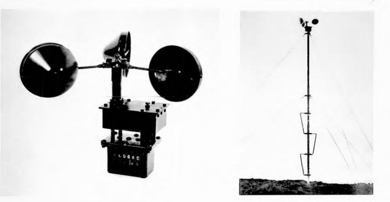
Fig. 27.—A modified cup-counter anemometer, Mk.2.
