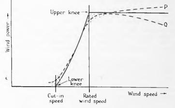
Fig. 19.—Power curves for steady and fluctuating winds.
